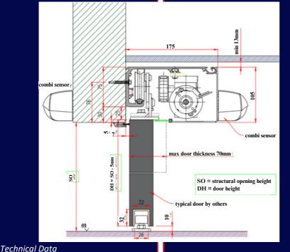
Power external devices 105x175mm Dimensions (h x d) 15V DC-12W Max 150 W Weight 11 kg/m **Rated Power** 1 wing: 70cm/s 2 wing: **Operating Temperature** -10oC > +55oC Maximum Opening Speed 140 cm/s Maximum Closing Speed IP rating IP20 70% of Opening Speed **SCAN ME!** Continuous Service Locking Electro-mechanical 1 Wing: 140 kg (HD 160kg) 230v AC 50/60Hz Maximum Payload 2 Wing: 100k+100g (HD Power supply 140k+140g 24 Vdc Motor with Power Unit Conformity CF integrated encoder
